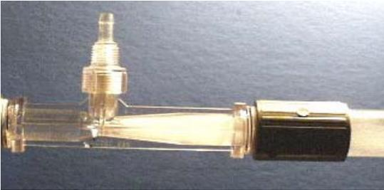
Injection equipment is necessary to facilitate effective dissolution of ozone into the process stream.
