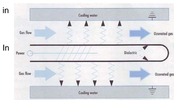
The collision of the electrons with the oxygen molecules in the introduced gas stream results in the formation of some ozone molecules. The amount of ozone formed is dependent on the characteristics of the electrical supply and the temperature of the treated gas.
