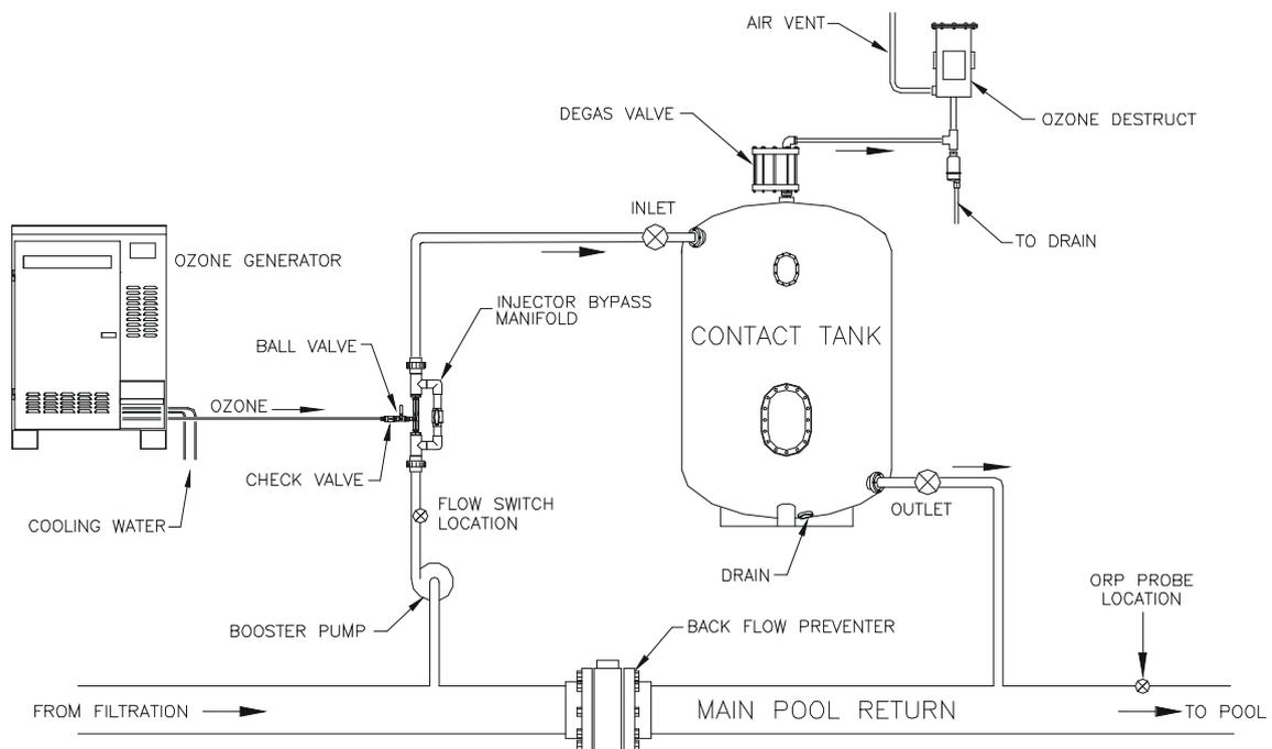
Figure 1: Sidestream ozonation system schematic diagram
