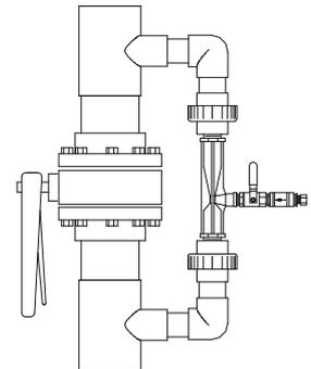
Figure-2: Venturi Injector Manifold
